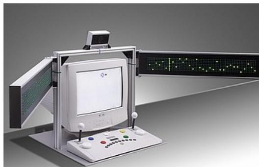
Image: The Vienna Test System with response panel and peripheral display panels.
